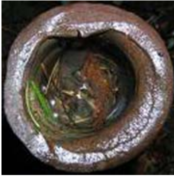
Figure 21. Looking down on an iron pipe corner. The edge is rolled from being hammered.
