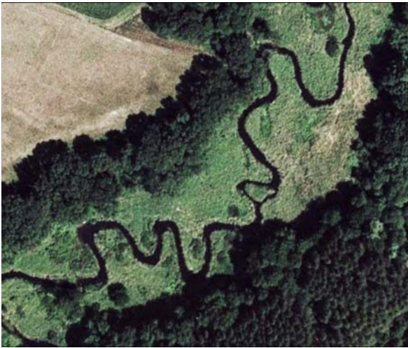
Figure 32a. A deed for an adjoining farm reads, "1045 ft to the top of bank," yet the river shown periodically shifts within the green "meander belt" by as much as 200-feet.
