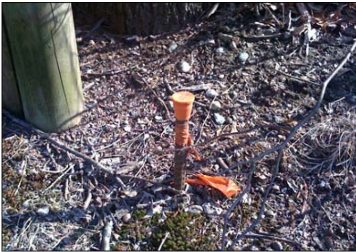
Figure 20. 3/4" iron rebar with plastic identification cap.
